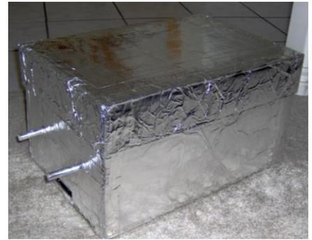
1. Cut two round holes in each side of the box a little more than half way up for the support rods. Cut two holes  $\frac{3}{4}$ " x 3-4" on each side close to the bottom to provide air for the charcoals.
