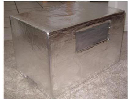
1. Cut out a 4x9" window at the top of the apple box if desired. Cut a 1x4" hole on the bottom of both ends of the box to allow air to get to the coals. Tape a piece of the plastic cooking bag over the window area. Cover box with aluminum foil inside and out. This works great by spraying box first with adhesive, attaching foil, and securing with the aluminum tape. Trick is to make sure that none of the cardboard is showing as it will burn.
